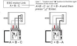
A+B-C or C+B-C must match the Initial Setup options of the Program Card. (WARNING! Improper configuration may damage the ESC.
